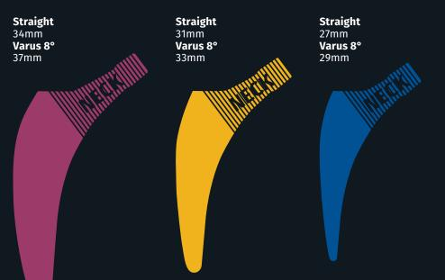
The clinical centroid is the driving force behind the Preserve design. A study of 900 radiographs, sampled globally, confirmed that femur size and neck length are positively correlated, and revealed that three neck groups is the optimal number for minimizing implant options while maximizing head center coverage and allowing for improved operating room flow. The design was robustly validated with an additional 150-case randomized templating study.
