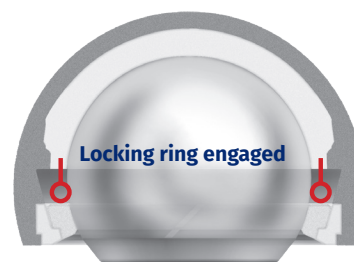
Head has been inserted. This causes the locking ring to engage and locks the head into place.
