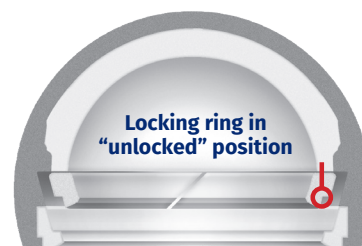
Locking ring in its "unlocked" position, without the head in the shell.
